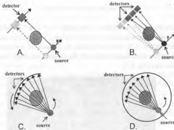
Fig. 1. The diagrams of the different CT scanners generations: A – the first-generation, B – the second-generation, C – the third-generation, D – the fourth-generation
