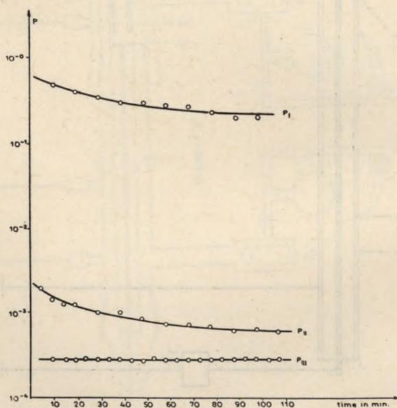
Fig. 3. Vacuum characteristics of the apparatus  $p_I$  — pressure in the chamber I,  $p_{II}$  — pressure in the chamber II,  $p_{III}$  — pressure in the chamber III
