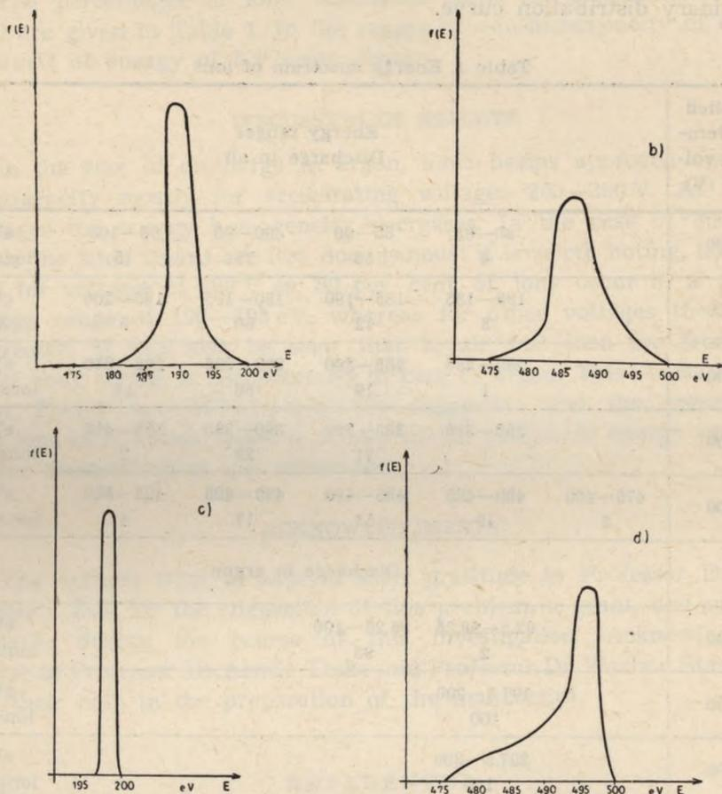
Fig. 10. Several typical energy distribution curves for accelerating voltages. Discharge in air a) 200 V, b) 500 V; discharge in argon, c) 200 V, d) 500 V. (The height of peak in Fig. 10 is given in a scale of 1:3 with respect to the remaining curves)
