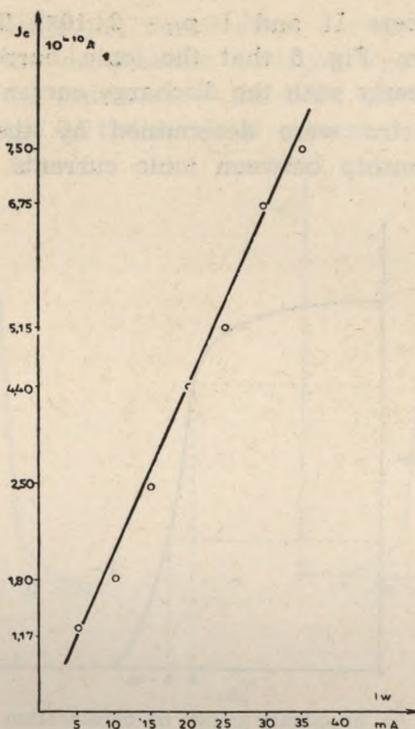
Fig. 6. The relation between ionic current  $I_c$  and the discharge current  $I_w$ .
