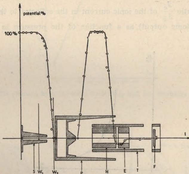
Fig. 4. Distribution of potential along the axis of the second and third chambers
