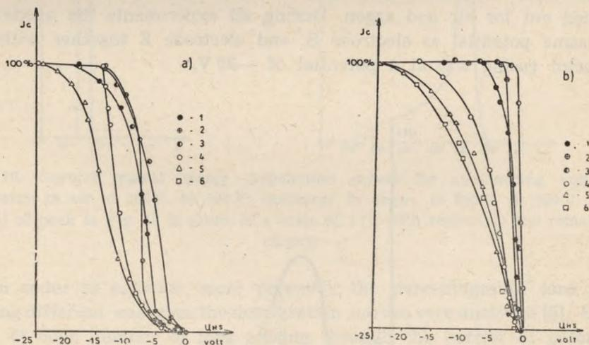
Fig. 7. Experimental decelerating curves for different acceleration voltages: 1 — 100 V, 2 — 200 V, 3 — 300 V, 4 — 400 V, 5 — 500 V, 6 — 600 V, a) discharge in air, b) discharge in argon
