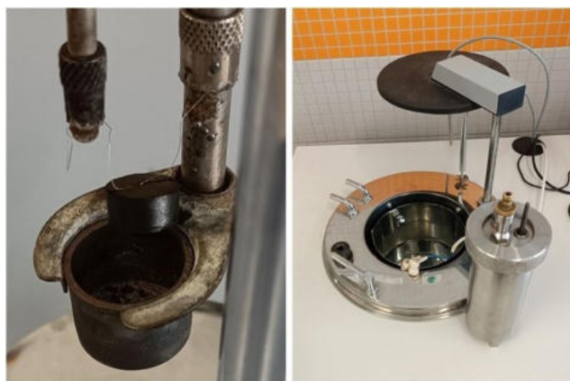
Figure 1. Compressed tablet connected to the electrodes (on the left) and the bomb calorimeter filled with oxygen (on the right).
